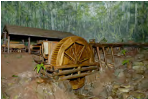
Scale model of the Curtis sawmill which was driven by a waterwheel
